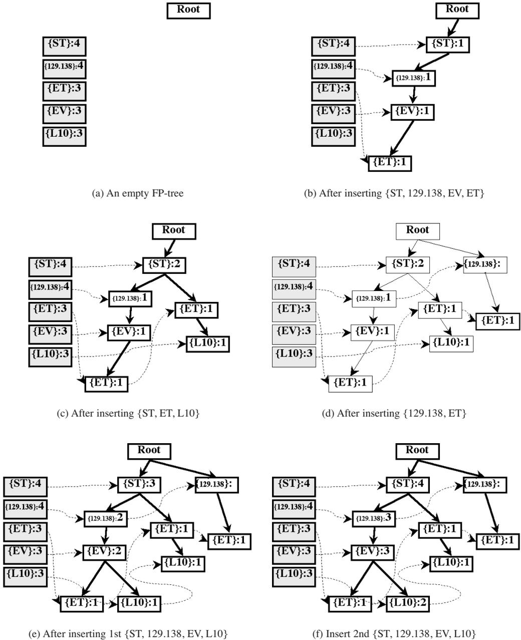
Figure 2: An example of an FP-tree construction
