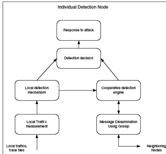
Figure 2: A conceptual architecture for an individual defence node
