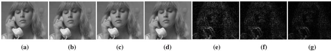
Figure 9: (a) *Suzie* frame #2, (b)–(d) Reconstructed frames using the H.264, Fixed-8, and EVPS(8, 75%) algorithms respectively, (e)–(g) Frame differences ( $\times 6$ ) of (b), (c), and (d) respectively with respect to (a)
